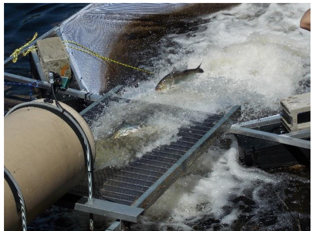
From Robert Stira of Firstlight and Power Resources: "It's from a survival test at the Scotland Fish Lift. The fish (shad) were tagged, released in the lift hopper and put through a lift cycle; the image was taken at the end of the cycle, at the discharge of the exit pipe. The fish were then held in a net pen for 24h for observation."
